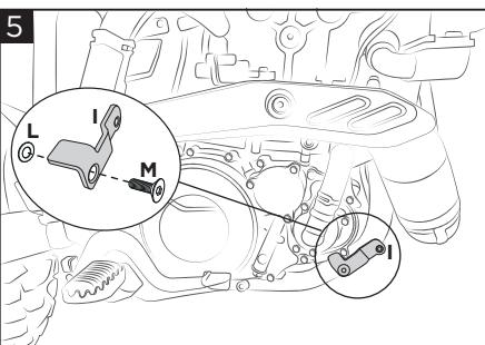
**Place the bracket (I) on the frame and secure it using the screw (M) and washer (L).**
