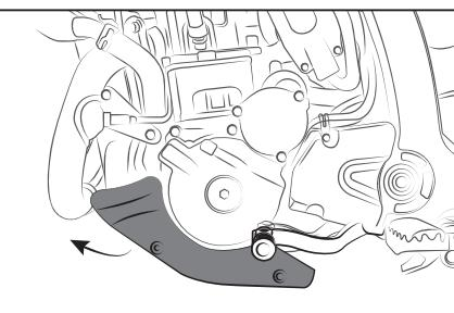
**Remove the original alluminium skid plate.**
