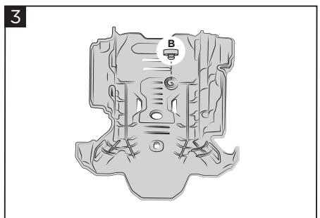
**Insert the grommet (B) into the appropriate seat on the Acerbis skid plate (A).**
