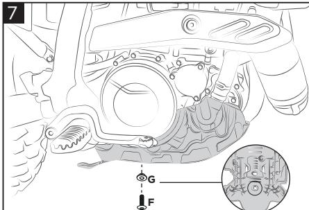
**Secure the rear part using the screw (F) and the bushing (G), without tightening.**
