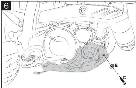
**Position the sub-motor and secure it with the screw (C) and the bushing (E) without tightening.**
