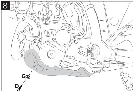
**Secure the left side using the screw (D) and the bushing (G) and tighten all the screws.**
